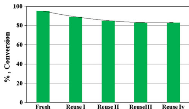
Fig. 12 Catalyst recycle study. Reaction conditions: methyl levulinate, 5 % (w/w); Solvent, MeOH (95 ml); H 2 pressure, 500 psi; temperature, 403 K; catalyst, 0.5 g (5 % Ru/C); reaction time, 2 h
